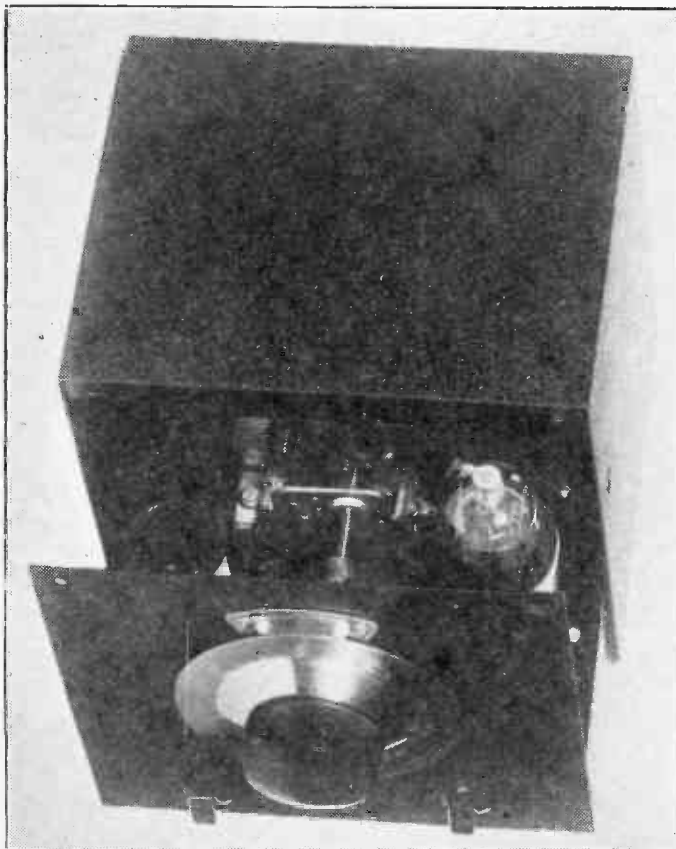
Built in a shield cabinet, the signal generator has a National precision dial. Calibrations are communicated to graph paper. The oscillator tube is a 34.
